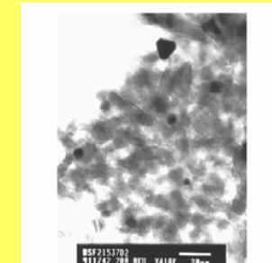
Automotive catalyst: 12 nm Pt on aged Al_2O_3
